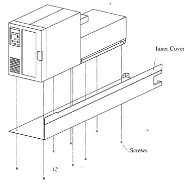
Figure 1-18. Mount FACL to Inner Cover
